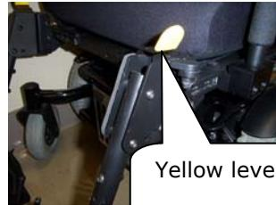
4. You can swing the control box to the side by pushing on the support and do the reverse to bring it back to its original position.
